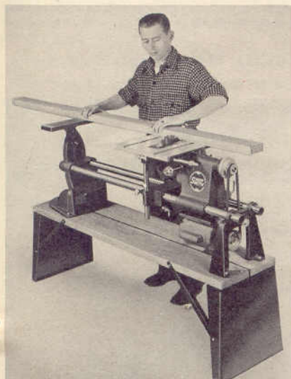
SHOPSMITH table extension makes it easy to do accurate work on long or bulky workpieces.
